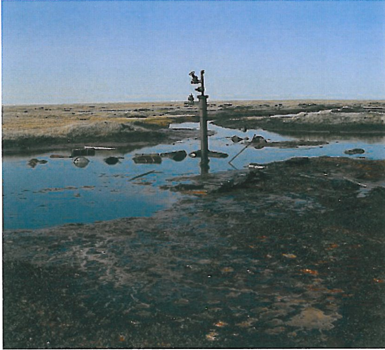
Simpson Core #26 drilled in the middle of an oil seep. Depth of the oily-water prohibits access to the wellhead.
